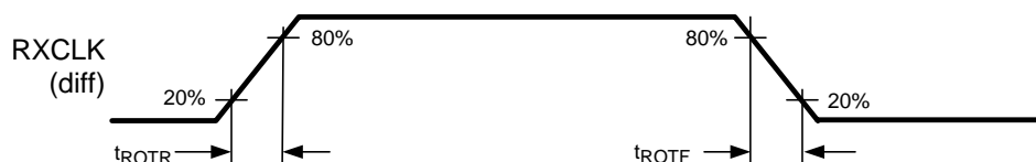
Figure 4. LVDS Output Transition Time
